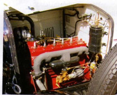
Continental Red Seal Motor. Six-Cylinder, side valve engine
